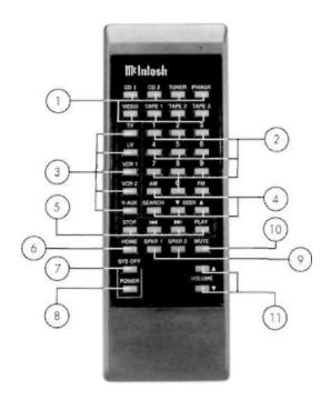
When using a Mcintosh CD Changer, the functions are STOP, BACK TRACK, NEXT TRACK and PLAY. In the STOP position, BACK TRACK selects which disc to play, and NEXT TRACK selects the SINGLE disc.
